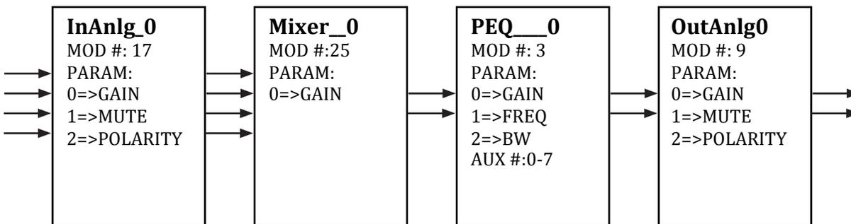
Similar concept as example #1, but this time the PEQ module is MOD #2 because the user added a 4 in-2 out mixer before it.
