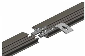
**Step 4.** After connecting the *center joints (e)*, insert 3 *brackets (g)* on each of the horizontal frames (top and bottom). Refer to the diagram below for *bracket (g)* placement. Note: The top and bottom center brackets will be used to secure the center support bar.
