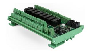
The ARU108MK2 is an intelligent relay unit featuring eight double pole relays with normal open and normal closed contacts. Control can be done through both digital (RS-485) and analogue (contact) input signals. Thanks to the flexible structure in terms of connectivity and control, the ARU108MK2 can be implemented in a wide variation of applications, adding flexible and intelligent functionality to your audio & video related or any other project.
