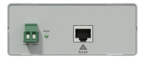
The rear panel of the APG20MK2 contains the 24 Volts DC input connection, together with the RJ45 bus input connection whereto the twisted pair bus cabling has to be connected.
