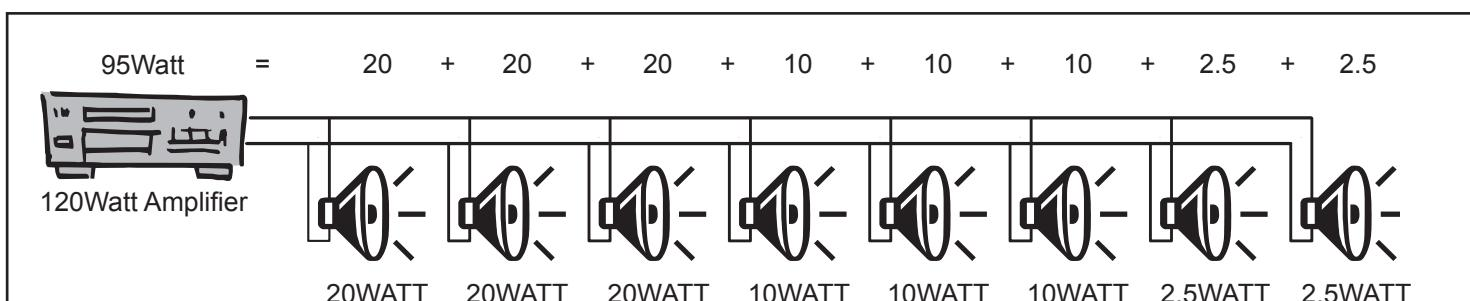
**Amplifier power must be higher than total power of all speakers.**
