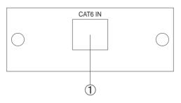
CAT6 IN: Connect from the CAT6 output of the transmitter with a CAT6 cable to the CAT6 input of the receiver.
