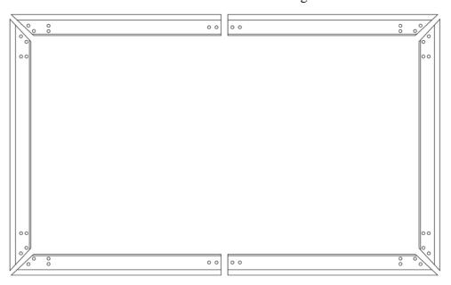
**Step 3.** Insert the *Center Joint (a)* connectors into one-half of the horizontal frame and secure with two 6x12mm Hex Screws (d). Once secure, connect the other half of the horizontal frame and fasten with two 6x12mm Hex Screws (d).
