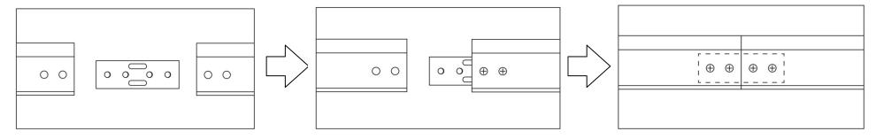
**Step 4.** Connect the *Elbow Joints* (*c*) to top and bottom sections of the vertical frame. Once inserted, connect the vertical sections to the horizontal frame sections. Make sure all the holes are in alignment and the frames pieces are flush (no gaps). They should form perfect right angles.
