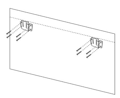
**Step 12.** Position the fixed frame screen onto the wall *Brackets* (g) as shown below and push down at the center of the top of the frame to secure.
