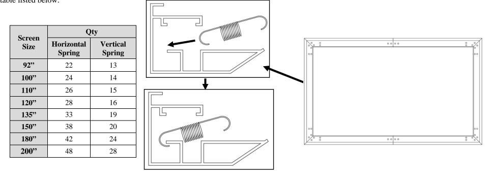
**Step 9.** With one end of the spring placed inside the groove of the frame, hook the *Spring (b)* through the hole located on the screen material's outer edge. **Be sure to hook the** *Springs (b)* **onto the** *Tension Rod (k)* **to avoid damage to the screen material.** Use the *Pull Hook (f)* when necessary. Attach the springs at the four corners (1).
