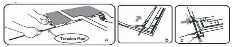
**Step 8.** Insert the *Springs (b)* into the grooves of the frame. Line them up with the corresponding holes in the materials edge. The shorter hook on each spring should be placed in the frame's groove, as shown below. For the correct amount of springs to place into the frame, please refer to the table listed below.
