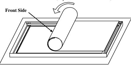
**Step 7.** Insert the four horizontal and two vertical *Tension Rods* (*k*) into the corresponding sides of the screen material, while keeping the material laying flat. Careful not to snag on the holes at the edge of the material during this process; forcing the rods may damage the screen material.
