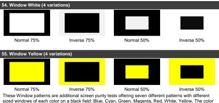
These Window patterns are additional screen purity tests offering seven different patterns with different sized windows of each color on a black field: Blue, Cyan, Green, Magenta, Red, White, Yellow. The colo patterns should display an even distribution of brightness and consistent color tone across the screen. Each pattern has 4 variations: Normal 75% Window, Inverse 75% Window, Normal 50% Window, and Inverse 50% Window.
