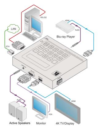
Figure 4: Connecting the 860 HDMI 18G Signal Generator & Analyzer
