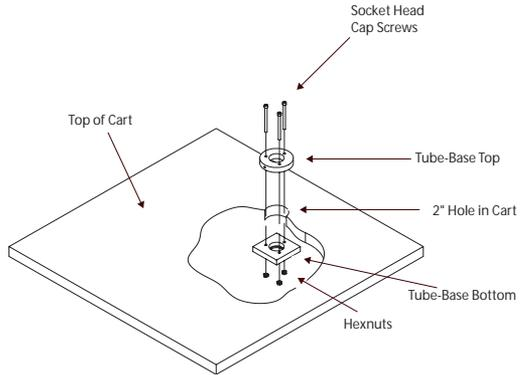
Figure 3.0 Tube-Base assembly
