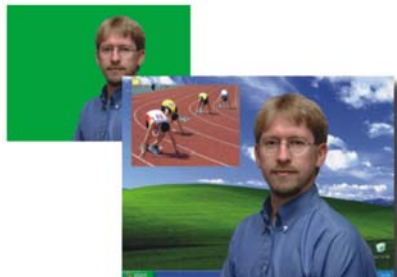
Dual Channel Chromakey with simultaneous PIP Insertion
