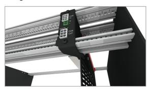
4. Screw the dock in place with two M3 screws.
