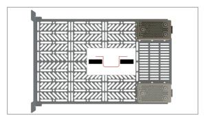
2. Turn the module over and screw the voltage selector in place with three M4 screws.
