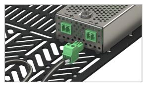
10. Use a long daisy-chain cable to connect the internal power supply to the module.
