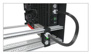
When you connect further modules, use the shorter daisy-chain cables to connect the output of the last dock to the input of the next dock.
