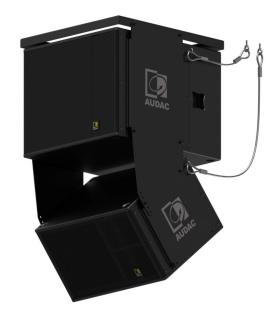
The MBK302S is a flying system for the FX series loudspeaker cabinets, allowing safe and stable mounting for one FX1.18 and FX3.15 to any type of ceiling or other supporting structure.
